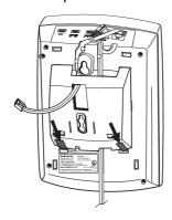
5. Plug the modular cord into the wall plate jack. Align the base's keyhole slots with the wall plate studs and slide the base downward to secure it.
